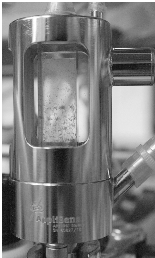
Fig. 2. Photo of the working ultrasonic resonator.
